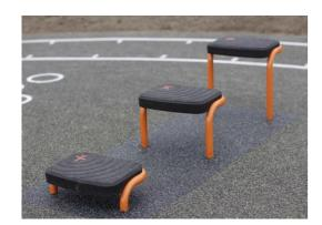
The support frame is ø48.3 x 4mm, carbon steel, with a hot-dip galvanised surface according to ISO1461, and a powder coating corrosion class C3 according to ISO12944-2. Lead content for surfaces is below 90ppm.
