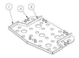
A 5 mm hot-dip galvanised carbon steel plate must is moulded inside the SBR to offer optimal stability and optimise the mounting of the step to the frame.
