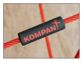
Corocord ropes with 19mm+ diameter are known as a 'Hercules' rope type which is formed from galvanised six-stranded steel wires. Each strand is tightly wrapped with PES yarn, which is melted onto each individual strand. Ropes are highly wear-and vandalism-resistant and can be easily replaced on-site if needed.
