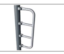
The FSW 209 features three 38 x 2mm push up bars at three heights of respectively 38cm, 58cm and 133cm.
