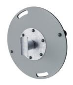
The bearing house is made from hot dip galvanised steel. The bearing shaft is made from stainless steel AISI304. The bearing itself is made from Polyoxymethylene (POM), an engineering thermoplastic with a high stiffness, low friction, and excellent dimensional stability.
