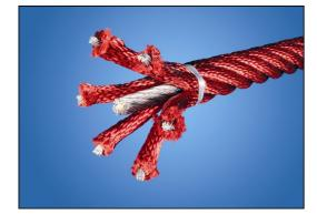
Corocord ropes of UV-stabilized PES rope strands with inner steel cable reinforcement. The polyester yarn is made from +95% postconsumer materials and is inductively melted onto each strand. PES has high strength with excellent resistance to abrasion and UV radiation. The ropes are connected by stainless steel S-Clamps which are pressed around the rope which results in a durable and vandalism solution, 2024
