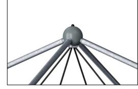
The unique designed connector balls with a diameter of 230mm are made of high quality aluminum with a powder coated top finish. The inside tensioning parts are made of hot dip galvanized steel.
