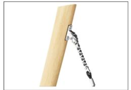
The swing hangers are made of stainless steel brackets and can move over two axis. The flange bearings are silicone enriched to make the suspension maintenance free. The connection to the rope is made with stainless steel chain.
