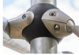
The unique designed GALAXY connection ball is made with an inner circular core of aluminium surrounded by a shell of hard PP with a outer layer of soft TPV rubber. Flexible lead free aluminium connectors allow for installation in variable angles.
