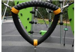
GALAXY climbing triangle with outer soft layer of PUR and corner brackets of moulded nylon (PA6). The core consist of a powder coated welded steel frame with integrated corner suspension points. Larger triangles are closed with an 18mm thick Ekogrip® panel that has a top-layer of rubber with a non-skid effect.
