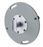
The bearing house is made from hot-dip galvanised steel. The bearing shaft is made from stainless steel AISI304. The bearing itself is made from polyoxymethylene (POM), an engineering thermoplastic with high stiffness, low friction, and excellent dimensional stability.
