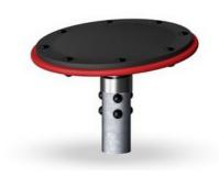
Upper plate is made of Ekogrip® panel that consist of a 15mm thick PE base with 3 mm top-layer of soft rubber with a non-skid effect.
