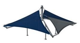
Sails of commercial 95 high density PE knitted specially for sun-shade structures. The sails are treated with UV stabilizers to ensure a long lifetime. The sails are supported by a hot dip galvanised steel frame and tightened by stainless steel devices.
