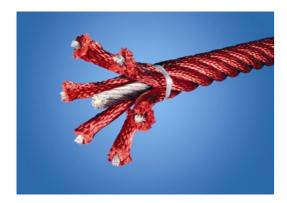
Saturn ropes has six-stranded steel wires and a steel wire core. Each strand is tightly wrapped with PES yarn, which is melted onto each individual strand and made from +95% Postconsumer Materials. After initial friction has removed the surface fibres, a harder PES coating remains to protect each strand, making the ropes highly wear- and vandalism-resistant.
