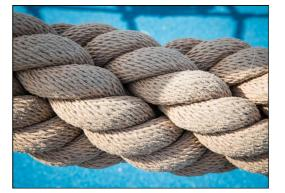
The PP rope in coconut style has a diameter of 150 mm. The internal steel wire core has thimbles at both ends, which serve as attachments for the rope to existing connecting elements.
