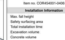
**Installation Information** 203 cm Safety surfacing area 60.2 m<sup>2</sup> Total installation time 30.5 Excavation volume 1.76 m<sup>3</sup> Concrete volume 0.98 m<sup>3</sup> Footing depth (standard) 90 cm Shipment weight 927 kg In-ground Anchoring options
