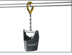
The sand bucket is made in one piece of molded PE. The PE is made with 33% postconsumer materials in different colors with a wall thickness of minimum 5mm. Material in accordance with the European Standard EN 71-3 and tested for UV stability.
