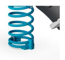
KOMPAN Springs are made of high quality spring steel according to EN10270. The springs are cleaned by phosphating before they are painted with an epoxy primer and a polyester powder coating as top finish. The springs are fixed by unique anti pinch fittings for maximum safety and long lifetime.
