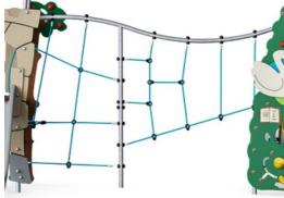
Climbing nets are made of UV-stabilized PP rope with inner steel cable reinforcement. The rope is induction treated to obtain maximum fixation between steel and rope which provides excellent wear and tear resistance. All rope connectors are made of 100% recyclable PA material.
