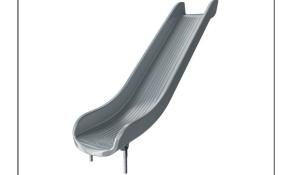
Molded PE slides made with 33% postconsumer materials in different colors in onepiece design with a wall thickness of minimum 5mm. The PE is tested for UV stability and has excellent impact strength and it is usable within a large temperature span.
