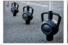
The tubes on which the magnetic bells move are ø40mm, made of grade AW 6082-T6 aluminium and have an anodized layer of  $20\mu$ m. The tube has a full steel core for structural integrity.
