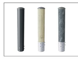
Main posts with hot dip galvanized steel footing are available in different materials: Pressure impregnated pine wood posts. Pre-galvanized inside and outside with powder coated top finish steel posts. Lead free aluminum with color anodized top finish. Greenline TexMade posts of 95% post-consumer recycled PE and textile waste.
