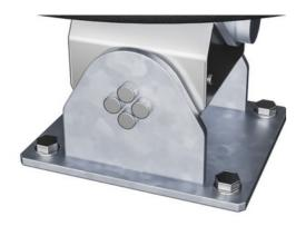
The double ROSTA element is made of ductile iron and has a hot-dip galvanized finish before painting. The ROSTA element is maintenance-free, with a elastic joint capable of a range of motion up to 250 degrees in any direction. Both wobbles have different stiffness, with a 45% disparity.
