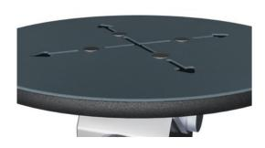
The ø414mm top plate is made from 15mm Ekogrip®, a 15mm PE plate with a 3mm top-layer of thermoplastic rubber with non-skid effect. The height is 217mm and the range of motion is +/- 90°, with a EPDM rubber stop at each end.
