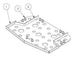
A 5 mm hot-dip galvanised carbon steel plate must is moulded inside the SBR to offer optimal stability and optimize the mounting of the step to the frame.
