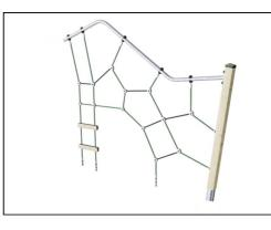
The rope nets are made of single braided 16 mm PES ropes. PES has high strength with excellent resistance to abrasion and UV radiation. The rope loops are assembled by aluminum connectors.
