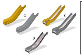
Slides are available in three different materials: moulded on piece PE slides, Combined EcoCore<sup>™</sup> sides and stainless steel slide bed t=2mm. Full stainless steel AISI304 t=2mm. The main posts are equipped with hot dip galvanised steel footings. The steel footings elevates the posts 20mm from ground level to avoid contact with surfacing material.
