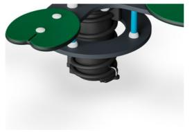
KOMPAN's springs are manufactured from highquality spring steel. The springs are cleaned by phosphating before being painted with epoxy primer and polyester powder coating. The springs are fixed by unique anti-pinch fittings for maximum safety and longevity.
