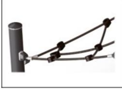
Rope loops of the seat are made of single braided 16 mm PES ropes. The polyester yarn is made from +95% post-consumer materials and is inductively melted onto each strand. PES has high strength with excellent resistance to abrasion and UV radiation. The rope loops are connected by nylon (PA6) connectors.
