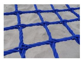
The nets for the hammocks are produced from 16 mm Corocord ropes. The connection between the ropes are manually spliced to avoid any hard objects in the lying area. The size of the meshsize does not allows to pass through the net.
