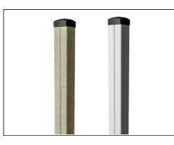
The main tower posts are available in two types of material: European pine wood posts, pressure impregnated Class 3 with Tanalith E3475 according to EN335 (Equivalent to NTR Class AB). Aluminum post t=2mm with anodized surface treatment. Base material EN AW-6060 T66.
