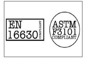
All KOMPAN fitness products are compliant with the ASTM F3101 & EN16630 Outdoor Fitness Standards. Load tests are performed as a static test by adding dynamic factors as well as safety factors to the specified load of 78kg per user. A product intended for 1 user is loaded with 420kg. and a second
