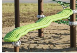
Rocking tube is made of medium density PE with excellent impact strength and usable within a large temperature span. Hollow plastic components are made of 100% recyclable PE made from 33% post-consumer materials. Molded in one piece with minimum 5mm wall thickness. The longitudinal grooves provides a slip resistant surface for safe play.
