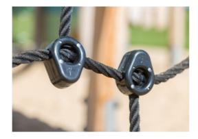
Ropes of UV-stabilized PES rope strands with inner steel cable reinforcement. The polyester yarn is made of +95% Post-consumer materials and is inductively melted onto each strand to obtain excellent wear and tear resistance.
