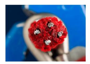
Corocord 16mm ropes are special 'Hercules'-type with galvanised four-stranded steel wires and a steel wire core. Each strand is tightly wrapped with PES yarn, which is melted onto individual strand. The ropes are hard wearing and vandalism resistant and are easy to replace for any given site.
