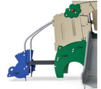
The steps are made of Ekogrip® panel that consist of a 15 mm thick PE base with 3mm top-layer of soft rubber with a non-skid effect. The steel surfaces are hot dip galvanized inside and outside with lead free zinc. The galvanization has excellent corrosion resistance in outside environments and requires low maintenance.
