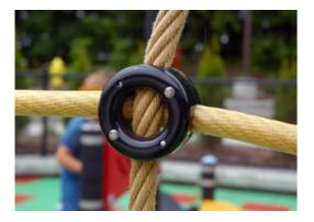
Climbing nets are made of UV-stabilised PA rope with inner steel cable reinforcement. The rope is induction treated to obtain maximum fixation between steel and rope which provides excellent wear and tear resistance. All rope connectors are made of 100% recyclable PA material. For installations using rubber surfacing the turnbuckle protectors are to be ordered separately.
