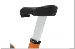
Seat is made of injection molded soft PUR with a powder coated steel inlay made from s235 steel. The user can choose between 9 different seat heights, ranging between 845mm and 995mm. The seat allows users with a height of 150cm to 195 cm to comfortably use the bike.
