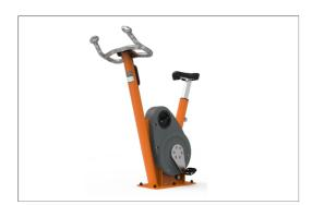
The from tube for the frame is made of S235 hot-dip galvanized steel tubing with the following dimensions Ø76,1x3,6mm. and with a powder coating corrosion class C3 according to ISO12944-2.
