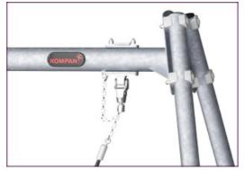
KOMPAN heavy duty designed swing hangers of stainless steel with anti-twist function. The moving parts of the swing hanger is lifetime sealed and lubricated. The hanger system is equipped with a safety chain to prevent the swing hanger to fall down if damaged.
