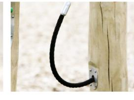
Ropes are made of UV-stabilized PA with inner steel cable reinforcement. The rope is induction treated in order to create a strong connection between steel and rope which leads to good wear resistance.
