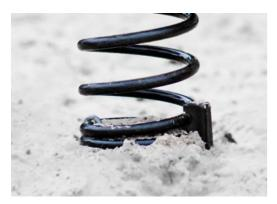
KOMPAN's springs are manufactured from highquality spring steel. The springs are cleaned by phosphating before being painted with epoxy primer and polyester powder coating. The springs are fixed by unique anti-pinch fittings for maximum safety and longevity.
