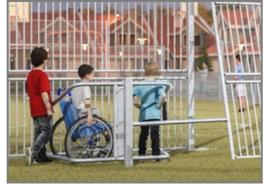
The wheelchair entrance is constructed of 80 x  $80 \times 3$ mm post with Ø 48mm tube and 2 stainless steel 16mm hinges. The opening is 95cm wide and 112cm long, this will allow people in a wheelchair to enter the MUGA but stops mopeds and motors.
