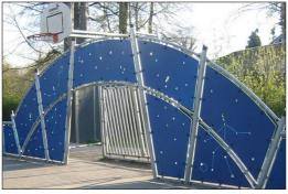
The goal measures ~140cm in depth and ~330cm in width, with all posts made of galvanized steel with a hot dip galvanized surface treatment. The front frame is made with Ø48 tubing, and the backside of the goal uses ten tubes with a diameter of ø38.
