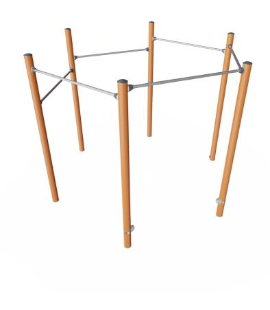
The hexagon pull up can be used in many ways and by multiple users at the same time. Exercises range from normal pull ups to the most dynamic and advanced exercises such as the Muscle Up. The pull up bars are made from solid steel and have a diameter of 32 mm. An ideal size for both men and women to have a good grip. As the highest bar is connected at a
