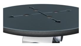
The ø414mm top plate is made from 15mm Ekogrip®, a 15mm PE plate with a 3mm toplayer of thermoplastic rubber with non-skid effect. The height is 217mm and the range of motion is  $+/-90^{\circ}$ , with a EPDM rubber stop at each end.
