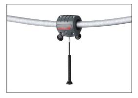
The hang-on puller is designed with at welded steel core and covered with low-density PE housing. The two hot dip galvanized steel handles are angled to provide best possible ergonomic while gliding. The wheels of the puller are made of low noise TPU and installed with sealed ball bearings.
