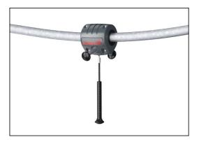
The hang-on puller is designed with at welded steel core and covered with low-density PE housing. The two hot dip galvanized steel handles are angled to provide best possible ergonomic while gliding. The wheels of the puller are made of low noise TPU and installed with sealed ball bearings.
