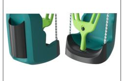
The front bumper is made with a core of strong polypropylene (PP) with a softer outer layer of thermoplastic rubber (TPE) and the rear bumper of 8mm thick EPDM membrane. The soft, shock absorbent bumpers with nonslip surface makes the swing seat extremely safe to use by caretakers.
