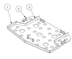
A 5 mm hot-dip galvanised carbon steel plate must is moulded inside the SBR to offer optimal stability and optimize the mounting of the step to the frame.
