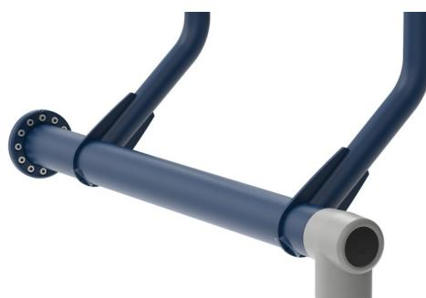
The input shaft is Ø101,3 x 2,9mm S355 Hot Dip Galvanized and Powder-coated steel. The bearing house is Caste Aluminum (EN AB-44100 / EN AB-AlSi12(a)) with self-aligning sealed ball bearings. An extremely strong and durable construction
