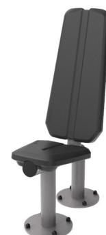
The seat is made of Polyurethane Rubber and has a steel insert plate that is electro-galvanized. The steel plate connects the seat to the frame. This construction makes the seat extremely durable against wear & tear and still very comfortable for a great user experience. The seat is positioned at a height of 46 cm, a comfortable height that makes the transfer from a wheelchair easy.
