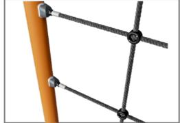
Corocord 16mm ropes are special 'Hercules'type with galvanised four-stranded steel wires and a steel wire core. Each strand is tightly wrapped with PES yarn, which is melted onto individual strand. The ropes are hard wearing and vandalism resistant and are easy to replace for any given site.
