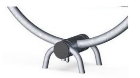
The rocking movement over axis is made by heavy duty scaled ROSTA torsion spring element. The ROSTA element works without any noise and requires low maintenance.
