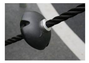
GALAXY ropes have six-stranded steel wires and a steel wire core. Each strand is tightly wrapped with PES yarn, which is melted onto each individual strand. After initial friction has been removed from the surface fibres, a harder PES coating is applied to protect each strand, making the ropes highly wearable and vandalism resistant.
