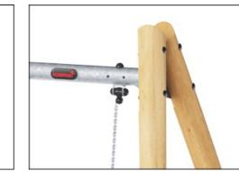
The swing hangers are made of high-quality UV-stabilised nylon (PA6) housing with integrated lifetime sealed ball bearings. The adjustable chains are fixed by a stainless steel hook with a theft-proof snake-eye bolt which is manufactured within an anti-twist house. All seats are fixed with two chains and are available with either standard or anti-wrap suspension.
