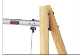
The swing hangers are made of high-quality UV-stabilised nylon (PA6) housing with integrated lifetime sealed ball bearings. The adjustable chains are fixed by a stainless steel hook with a theft-proof snake-eye bolt which is manufactured within an anti-twist house. All seats are fixed with two chains and are available with either standard or anti-wrap suspension.
